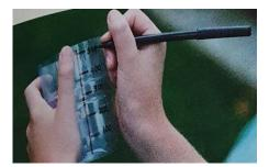
2. Mark the counter scale to 500 millimetres. Dig a small hole in the ground for the meter to keep it from tipping over and set it in, or attach the meter to a stand.
